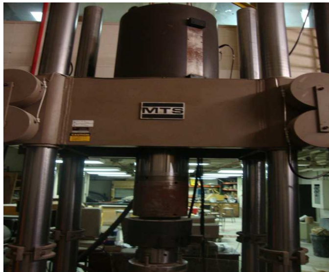
Figure 4.4: MTS 810 machine employed for compression test
